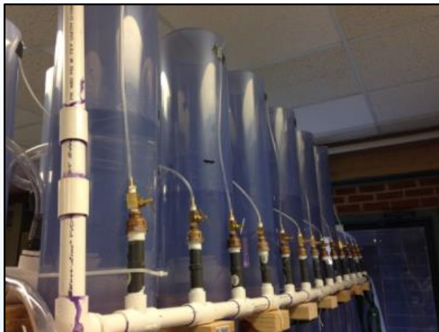
Bend in outflow tubing 18" above outlet elevation for static water level control
